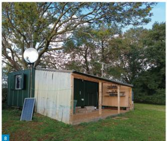
Fig. 6: The main mast supports a three-element beam for 6m, a two-element Tribander for 20m, 15m and 10m, and other wire antennas. Fig. 7: A drone's-eye view of the beams. The shack can be seen in the distance below. (Photo: Nick Garrod). Fig. 8: The shack and veranda. The dish and Yagis are for satellite work and the solar panel in the foreground provides a 12V supply for ancillaries. Fig. 9: Dan finds his 3D printer ideal for manufacturing small antenna accessories.
