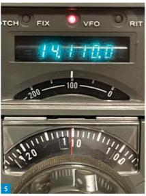
lower analogue display changes as the dial rotates each 100kHz segment. It's a joy to see although a bit fiddly to adjust and service.
