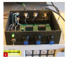
with a receiver, omitting the PTT circuitry. This worked wonderfully well so I built another three, all combined within one case, to serve three other receivers. I then bought a damaged SEM QRM Eliminator off eBay for not a lot, repaired it, and added it to another receiver.
