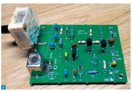
The other method of testing is to simply listen for the oscillator's signal on an SSB receiver covering the intended frequency. If you attached an 'aerial' wire about 30cm long to the VFO's RF output, you should be able to hear the radiated signal using a nearby receiver. You won't be able to measure the RF volts using this method but it does allow you to set the frequency range, and calibrate the VFO.
