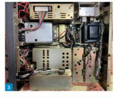
up to see if anything worked. I was encouraged to find that at 12V it was drawing about 1.6A, which matched the supply current documented in the manual. There is no internal speaker so I connected an external speaker and antenna wire and was delighted to find that the receiver seemed to work to some extent.
